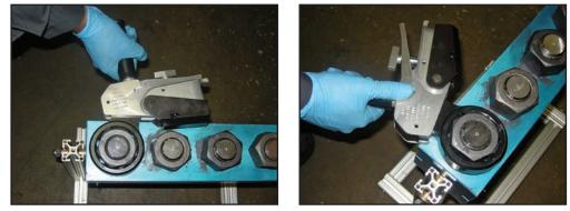
When loose, the wrench can be removed from the nut.
